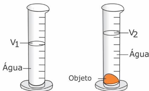
$$\text{Volume do objeto} = V_2 - V_1 \quad 4$$
