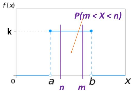
$$\text{Área} = \text{base} \times \text{altura} = (m - n) \times k$$
