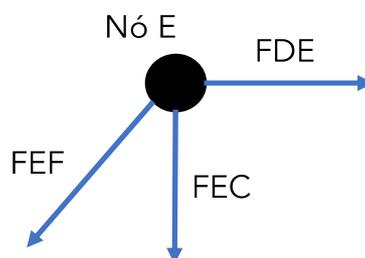
$$\begin{aligned}\sum F_x = 0 &\Rightarrow FDE - FEF_x = 0 \Rightarrow FEF_x = 20 \text{ kN. (T)} \\ \sum F_y = 0 &\Rightarrow -FEC - FEF_y = 0 \Rightarrow -FEC - \left(\frac{FEF_x}{\cos 45^\circ} \cdot \cos 45^\circ\right) = 0 \Rightarrow FEC = -20 \text{ kN (C)}\end{aligned}$$
