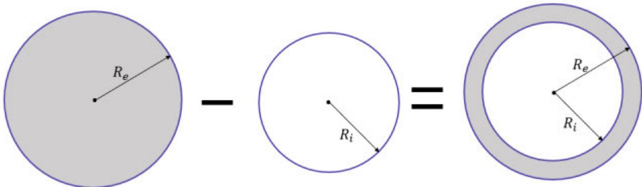
$$A_{coroa} = A_{externo} - A_{interno} \rightarrow A_{coroa} = \pi R_e^2 - \pi R_i^2 \rightarrow A_{coroa} = \pi(R_e^2 - R_i^2)$$
