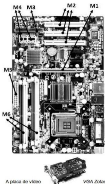
GeForce GTX660 2GB DDR5 192-Bit PCI-Express 3.0 x16 SLI Support - ZT-60901-10M #Daylight offboard deve ser instalada no slot identificado por:
