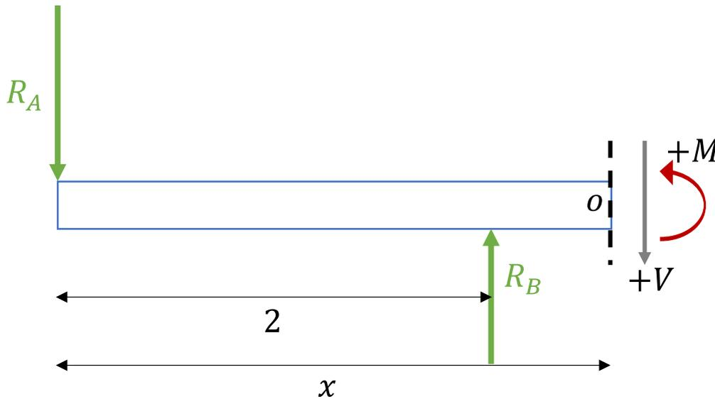
$$\sum M_O = 0 \quad M + R_A \cdot x - R_B \cdot (x - 2) = 0 \Rightarrow M = R_B \cdot x - R_B \cdot 2 - R_A \cdot x$$
