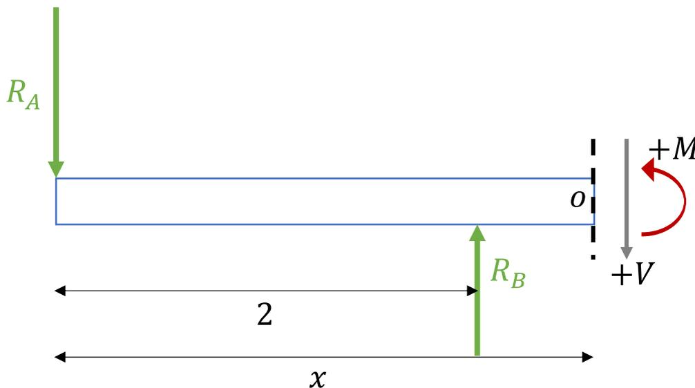
$$\overset{+}{\curvearrowright} \sum M_O = 0 \quad M + R_A \cdot x - R_B \cdot (x - 2) = 0 \Rightarrow M = R_B \cdot x - R_B \cdot 2 - R_A \cdot x$$
