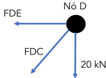
$$\begin{aligned}\sum F_y = 0 &\Rightarrow -20 \text{ kN} - FDC_y = 0 \Rightarrow FDC_y = -20 \text{ kN (C)} \\ \sum F_x = 0 &\Rightarrow -FDC_x - FDE = 0 \Rightarrow -\left(\frac{FDC_y}{\cos 45^\circ} \cdot \cos 45^\circ\right) - FDE = 0 \\ &\Rightarrow -\left(\frac{-20 \text{ kN}}{\cos 45^\circ} \cdot \cos 45^\circ\right) - FDE = 0 \Rightarrow FDE = 20 \text{ kN (T)}\end{aligned}$$
