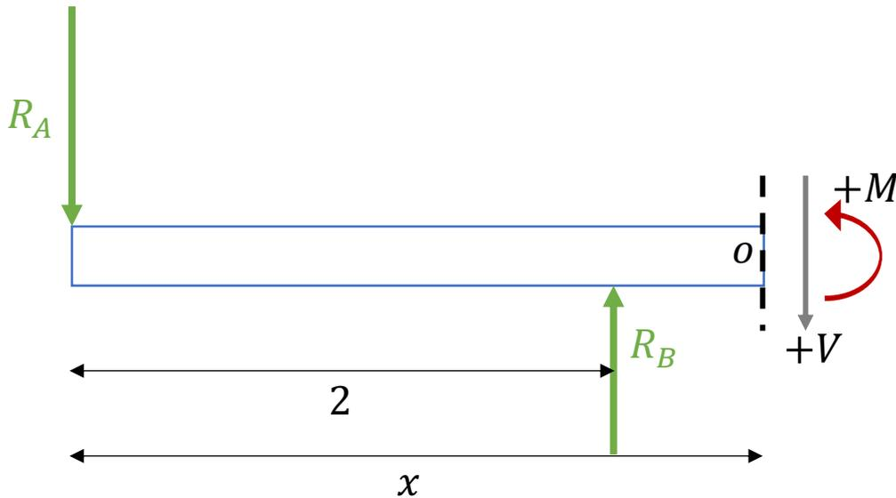
$$\sum_{\circlearrowleft} M_o = 0 \quad M + R_A \cdot x - R_B \cdot (x - 2) = 0 \Rightarrow M = R_B \cdot x - R_B \cdot 2 - R_A \cdot x$$
